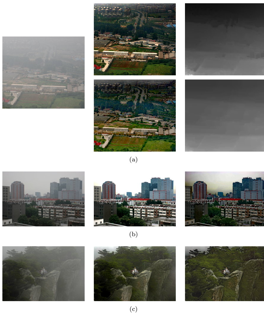
Fig. 9 Factorization results of real-world foggy images, of (a) an aerial city view, (b) an urban view, and (c) a cliff, compared with those of another method by He et al (2009b). For the example in (a), in the columns, the input foggy image (left), the estimated albedo image (middle), and the estimated depth image (right) are shown; and in the rows, the results by He et al (2009b) (top), and by our method (bottom) are shown. For the examples in (b) and (c), the input image, the albedo image by He et al (2009b), and the albedo image by our method are shown from left to right, respectively. Overall the factorization results are of similar quality, but our method achieves clearer defogging on particularly challenging scenes like that in (c). Occasionally our EM method may favor the depth prior and result in artifacts such as the trees in (a). The input images and the corresponding results by He et al (2009b) are reprinted from (He et al, 2009a).
